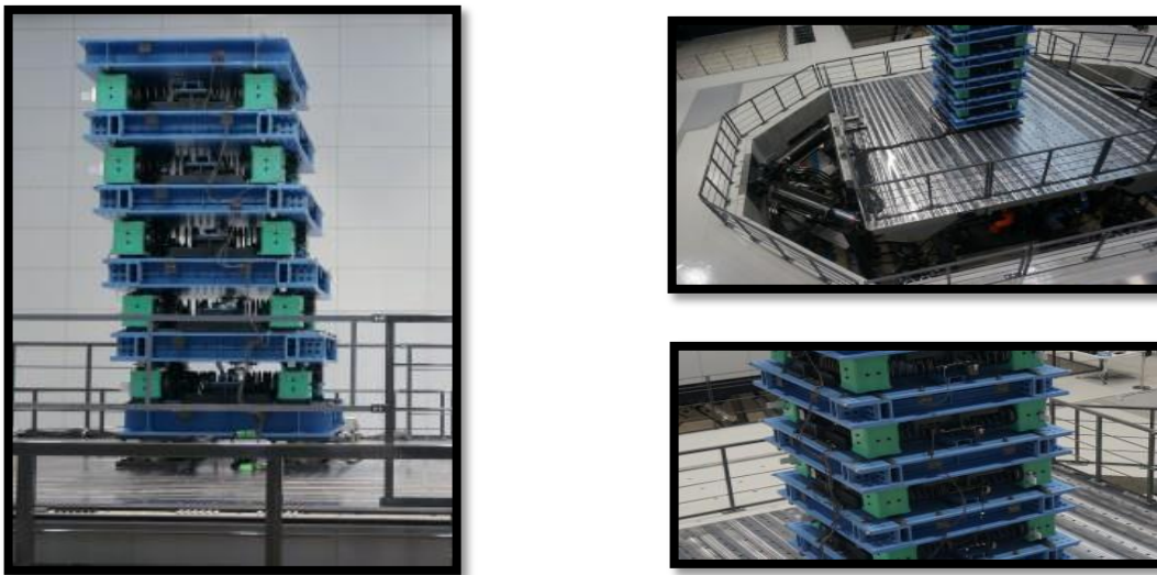
FIG 14.2: EXPERIMENT USING E-BEETLE (LARGE-SCALE SHAKING TABLE)
