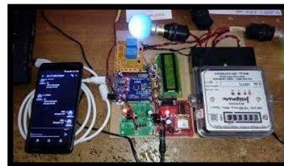
FIG 8.6: REMOTE MONITORING AND CONTROL OF DIGITAL ENERGY METER
