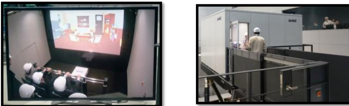
FIG 14.3: EARTHQUAKE SIMULATIONS USING THE E-SPIDER (LARGE-STROKE SHAKING TABLE)
